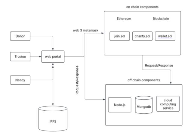
Fig. 4.1: System architecture
