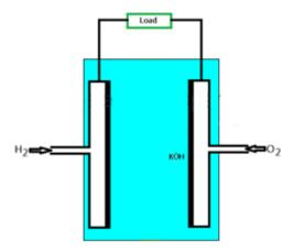
The electrodes are made up of sintered Nickel plates having a coarse pores surface and a fine pores surface; the two surfaces for gas and electrolyte respectively. A solution of KOH is used as electrolyte. The water vapor formed during the reaction is passed back by condensation from the opening for passing hydrogen into the cell.
