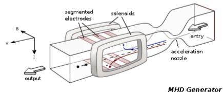
Faraday linear nozzle with segmented electrodes
