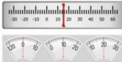
Moving scale with fixed pointers
