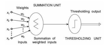
Here,  $x_1$ ,  $x_2$ ,  $x_3$ , ...,  $x_n$  are the n inputs to the artificial neuron.  $w_1$ ,  $w_2$ , ...,  $w_n$  are the weights attached to the input links.
