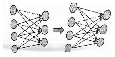
DropConnect has been proposed to add more noise to the network. The primary difference is that instead of randomly dropping the output of the neurons, we randomly drop the connection between neurons.
