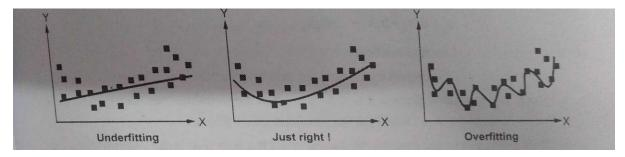
Just have a look at the above figure, and we can immediately predict that once we try to cover every minutest feature of the input data, there can be irregularities in the extracted features, which can introduce noise in the output. This is referred to as "Overfitting".
