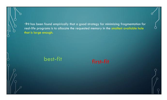
→ To implement best-fit placement more efficiently, we can separate free space into bins, according to their sizes.
